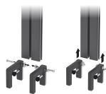
Make sure the nut and bolt are loosely screwed together on each
