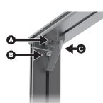
Tighten bracket attachment screws A
